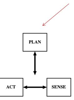
The robot first plans (deliberates) how to best decompose a task into subtasks (also called "mission planning").
