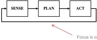
Focus is on planning: at each step, the robot explicitly plans the next move
