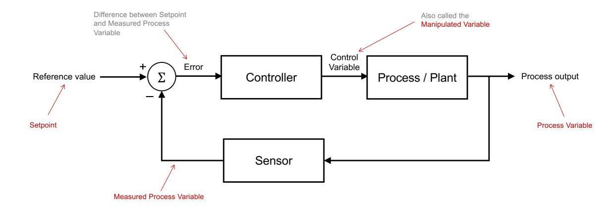
For example, controlling the orientation of a mobile robot
