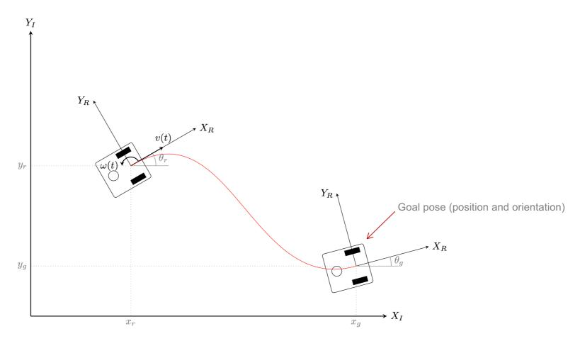
For example, controlling the orientation of a mobile robot
