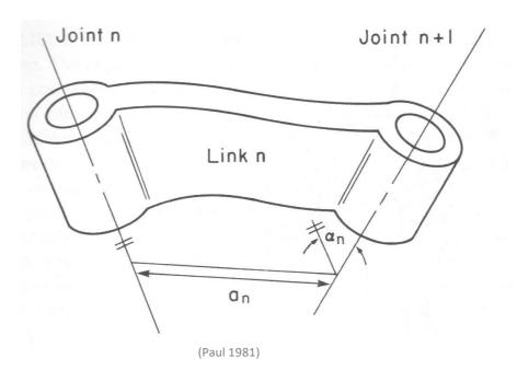
Link **length** (common normal distance)  $a_n$ Link **twist** (angle between the two axes)  $\alpha_n$
