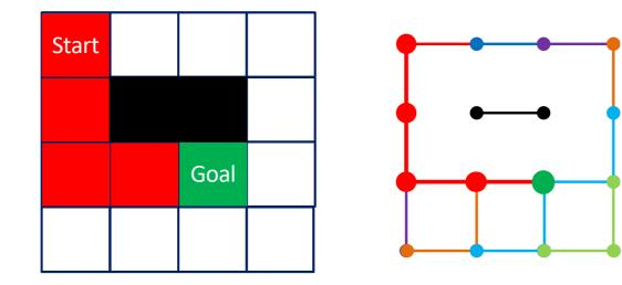
If required, mark the path from the robot start position to the goal position on the occupancy grid (value = 2)
