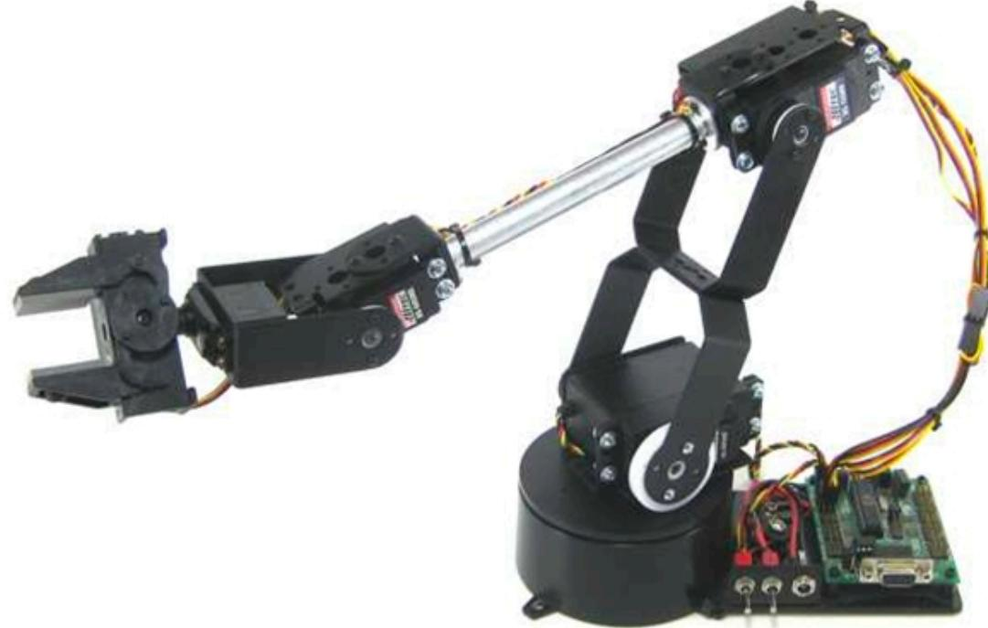
Lynxmotion AL5D Robotic Arm with serial interface
