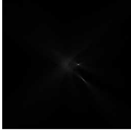
Figure 3.6. Hough transform of the image sequence in fig 3.5; the velocities of the component images correspond to the positions of the two maxima.
