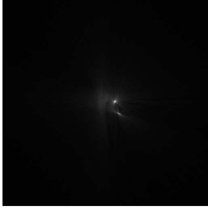
Figure 4.5. Hough transform of the image sequence in fig 4.4; the velocities of the component images correspond to the positions of the two maxima.
