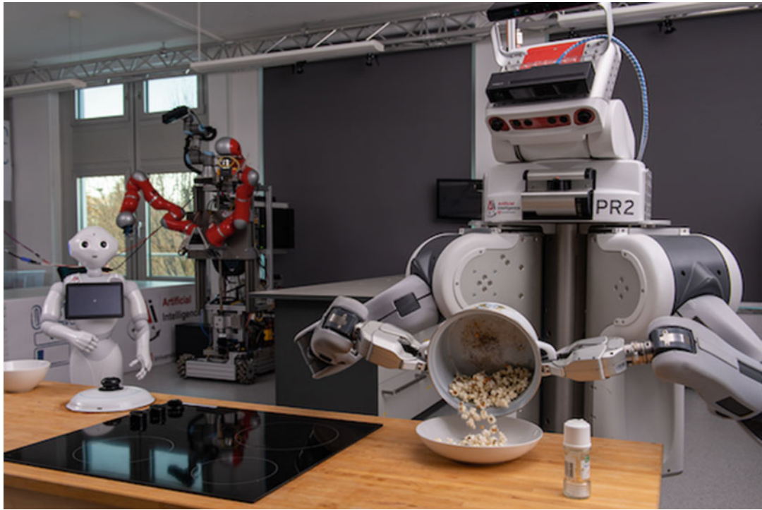
Cognitive Robotics, Fig. 2 A PR2 robot demonstrating cognition-enabled manipulation by using knowledge and reasoning to determine the motions required to pour popcorn from a saucepan
