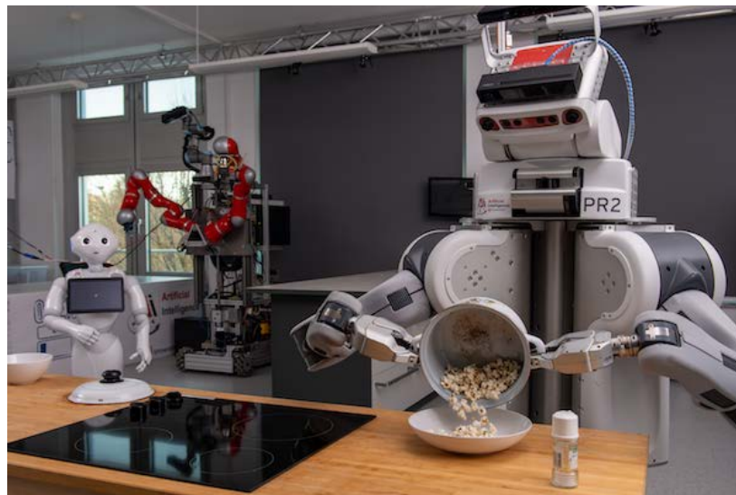
Fig. 2. A PR2 robot demonstrating cognition-enabled manipulation by using knowledge and reasoning to determine the motions required to pour popcorn from a saucepan.
