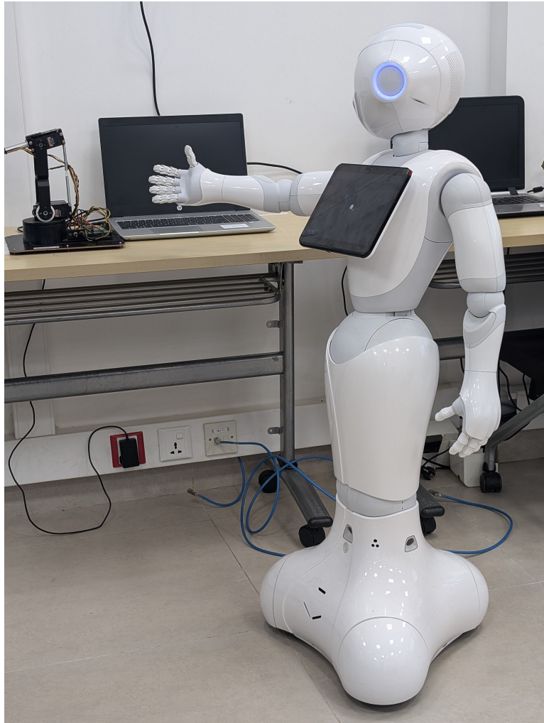
Fig. 2: The Pepper robot performing a deictic pointing gesture during the experiment. Note that the robot's gaze is directed to the object to which it is gesturing. The picture is taken from the perspective of the user in the study.
