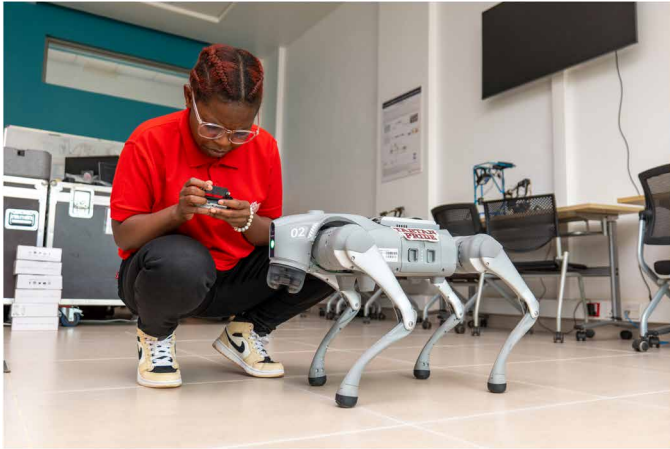
Melinda Mudzurandende, a student at Carnegie Mellon University Africa, working on a project to equip a Uniree Go2 quadruped robot with the ability to learn how to act by observing how other agents act.
