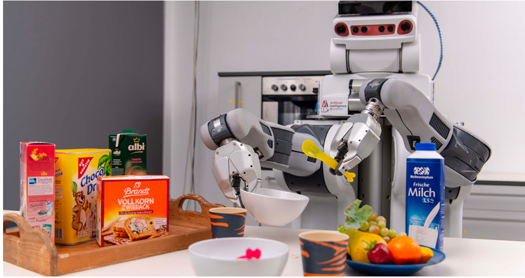
Figure 10.1: A PR2 robot setting a table during a demonstration of cognition-enabled robot manipulation using CRAM (image courtesy of the EASE interdisciplinary research center at the University of Bremen, Germany).
